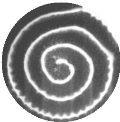
FIG. 12. A one-armed spiral showing an oscillatory instability. This image was taken in a flat-bottomed cell with N=25 , f=22 Hz, and \Gamma=3.30 .
